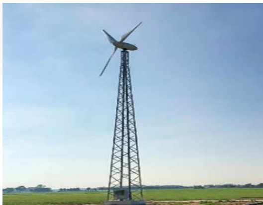
Figure 3.3: Ryse Energy E-10 10 kW wind turbine, and its power curve [41].
